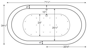
Requires use of a wall-mounted or freestanding tub filler. The drain and overflow assembly is concealed between the walls of the tub, eliminating the need for an exposed drain kit.
